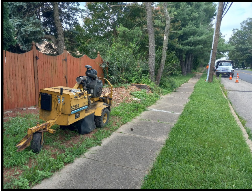
Photograph 6 – Tree subcontractor preparing to grind stump of fallen trees.
