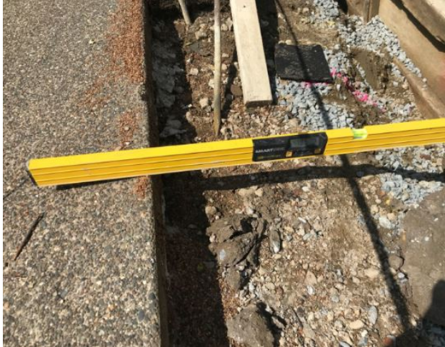
Figure 4: Concrete driveway slope measurement
