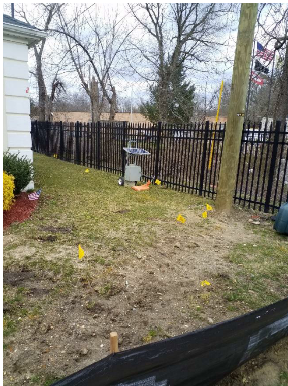
Seismograph has been put in place to monitor and vibrations caused by the Construction activities
